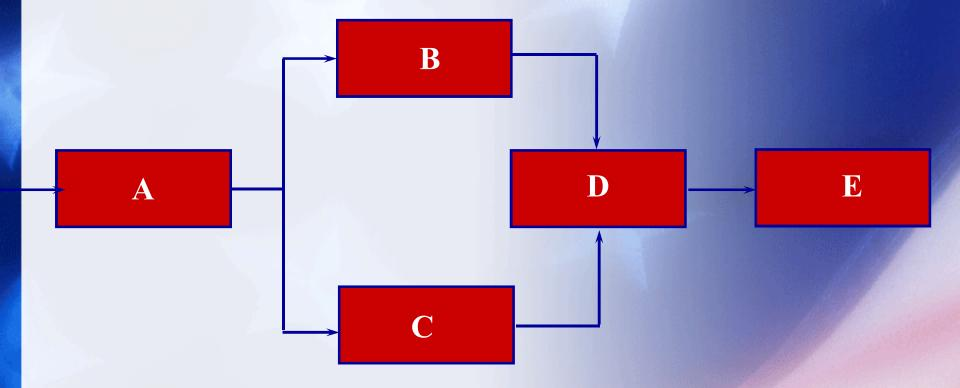
Success Space: An input signal to A provides an output to B and C. An output from B and/or C produces a signal from D which finally passes a signal to E.
