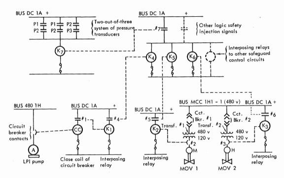
Fig. 2. The LPIS control circuit: The ECCS, including the LPIS, is actuated by a safety injection signal (SIS). The LOCA creates conditions such as "low-pressurizer water level" and "low-pressurizer pressure" that are detectable by transducers. For simplicity, the actuation of the LPIS is described for the case when the SIS is generated from the two-out-of-three circuit for high containment pressure.
