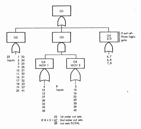
Fig. 4. Boolean equivalent of the LPIS fault tree.
