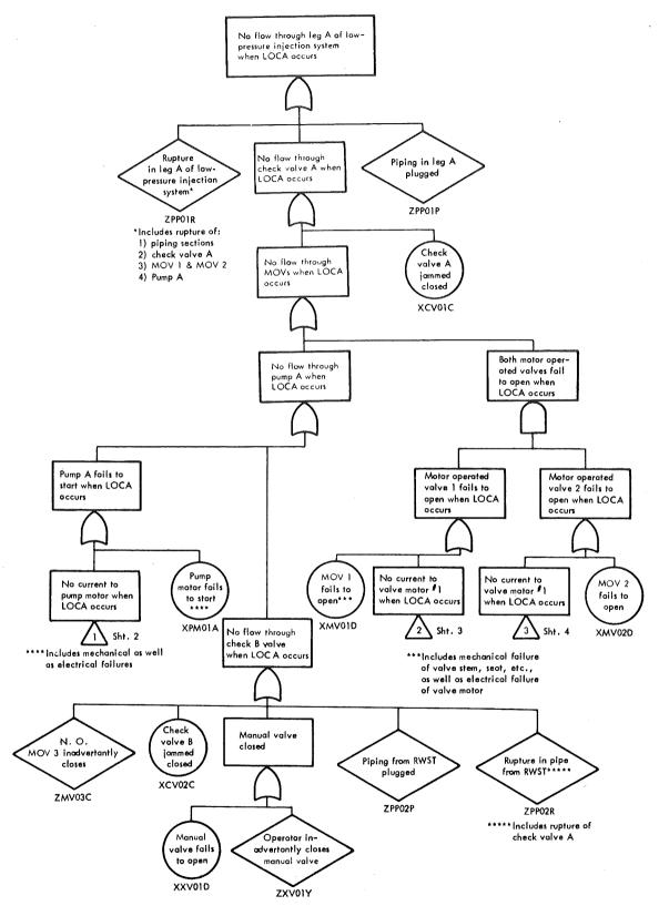
Fig. 3. Fault tree for the LPIS.
