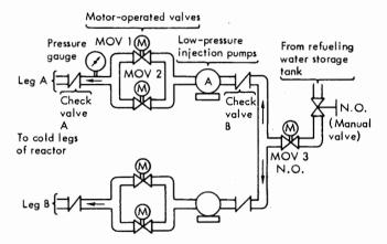
Fig. 1. Low-pressure injection system.
