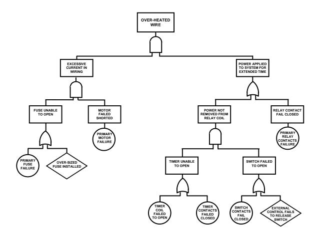
FIGURE 6: FAULT TREE WITH PRIMARY FAILURE TECHNIQUE
